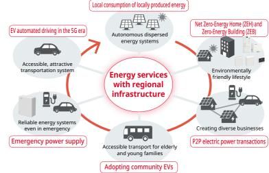
\* P2P-based power transaction: Power supplied by individual and/or corporate owners of solar power generators, storage batteries, and related renewable facilities is optimized to meet fluctuating user demand via AI-driven predictive analytics and other technologies
